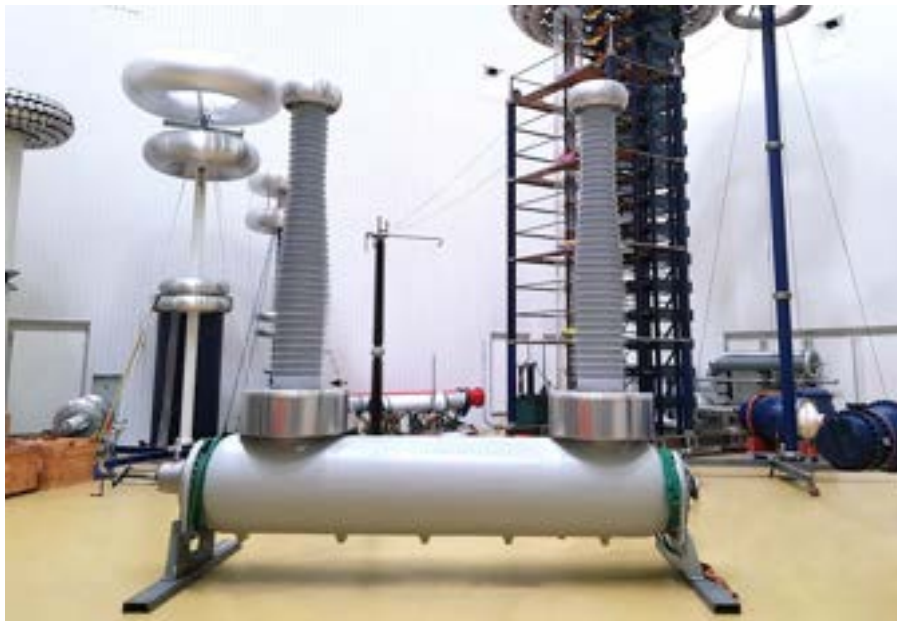
DTB version in high voltage testing
