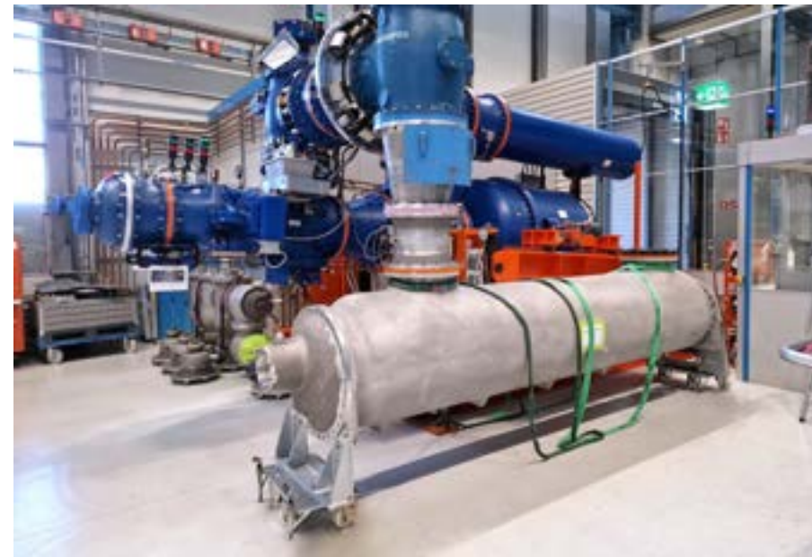
GIS version at factory routine test facility
