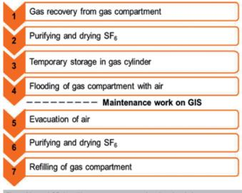
Fig. 1: Normal  $\mathrm{SF}_{\rm 6}$  handling sequence on gas insulated switchgear Source: DILO
