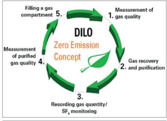
Fig. 2: DILO's Zero Emission Concept and its steps
