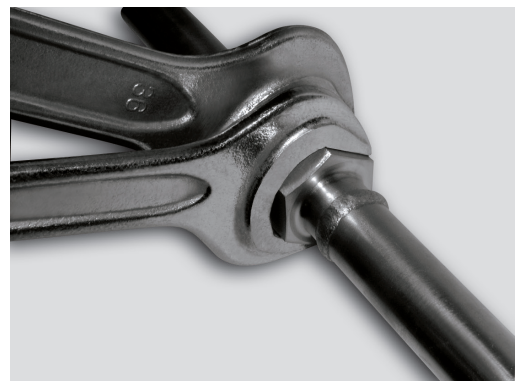
10. Observe the lubricating points of lubricant at a DILO tube union.
