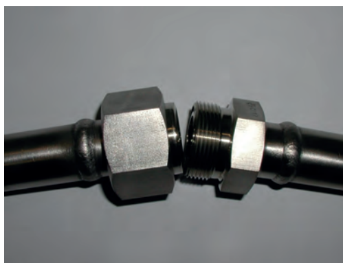
6. Wrong: not properly aligned welded tube union results in leakage
