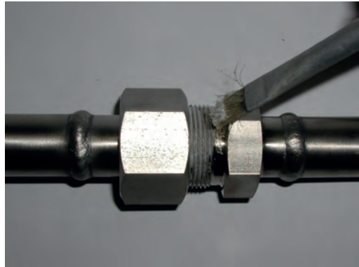
8. Lubricate - especially the austenitic steel - with suitable lubricants (e. g. type Never Seez from -180^{\circ}\text{C} to +1,400^{\circ}\text{C} / order no. 05-1172-R001)
