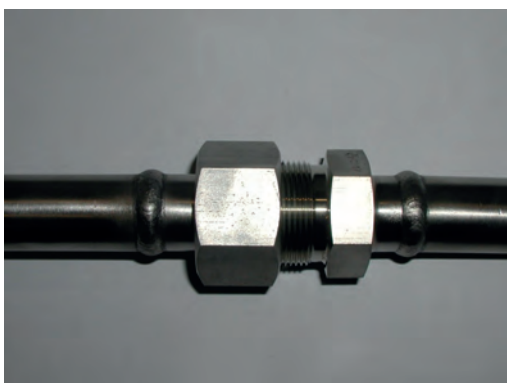
5. Right: aligned welded tube union
