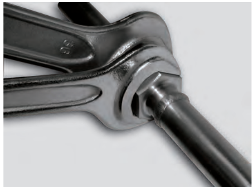
10. Tighten the clamping nut taking into consideration the specified torque by counteracting force.
