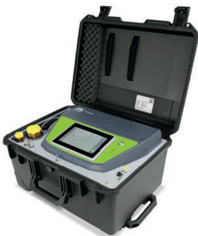
Figure 1: MultiAnalyser for measuring concentration of C4-FN or C5-FK, oxygen (O 2 ), moisture (using electr. dew point sensor), carbon dioxide (CO 2 ) and carbon monoxide fraction (CO).
