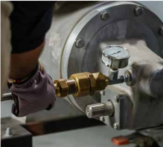
Self sealing fittings reduces gas handling emissions
