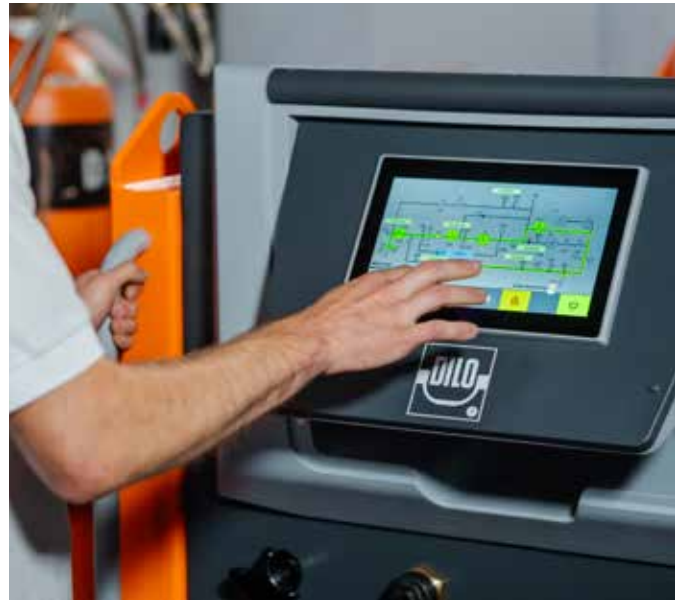
Gas recovery equipment designed for emission free gas handling
