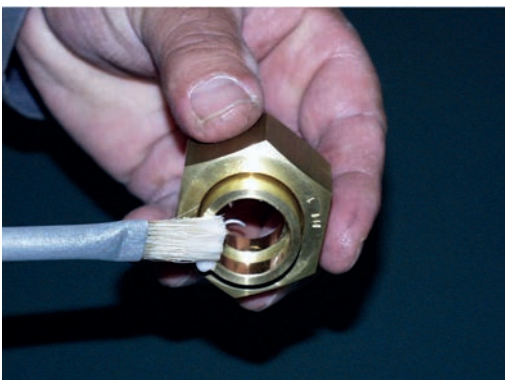
5. Apply the soldering flux at the part to be soldered
