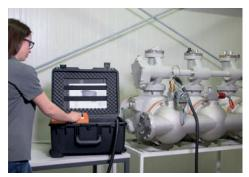
In combination with a special lock valve the DensiControl IN density monitor testing device allows reliable verification of density monitors directly on the gas compartment.
