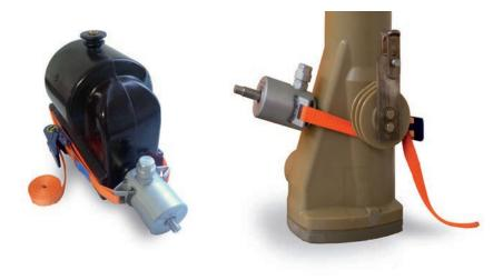
Prior to the gas recovery process the gastight cutting device can be mounted on the medium voltage components by means of a ratchet strap.
