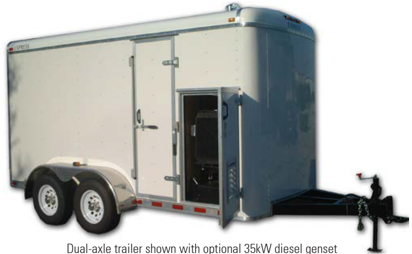
Dual-axle trailer shown with optional 35kW diesel genset
