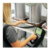
The measuring sensor extension (included in the scope of supply), which can be installed between the device and the measuring sensor, if necessary, allows measurements on measuring points difficult to access.
