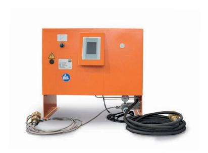
For the measurement, the gas compartment is equipped with two partially separated couplings. The gas is taken from one of the two couplings, temporarily stored in the internal gas collecting bag of the gas monitoring system and then pumped back into the gas compartment through the second coupling after the measurement has been taken. Alternatively, the gas outlet coupling of the device can also be connected to an external vessel where the gas is collected after the measurement.
